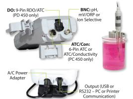
12 mm and 16 mm probes can utilize the **Grip-Clip™** to attach one or more sensors to a beaker and to the instrument as needed. The stand can be extended as shown above or used for wall-mounting.
