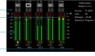
When the Dolby E decoder is selected as the metering source (ST 2110, SDI or 2022-6 mode), the view of the analyzer changes to display the 8 channels of decoded Dolby E audio as well as the stereo 2.0 downmix
