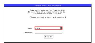
Using the User Login feature allows the Sx to be protected from unauthorized operation of the Front Panel controls. The prompt feature can allow a message to be displayed so that if the Sx instrument gets lost or stolen, someone finding it knows where to return it.
