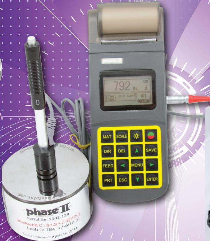
The PHT-3500 can perform tests that easily convert to the most popular hardness scales, including Rockwell, Brinell, Vickers, Shore, etc.
