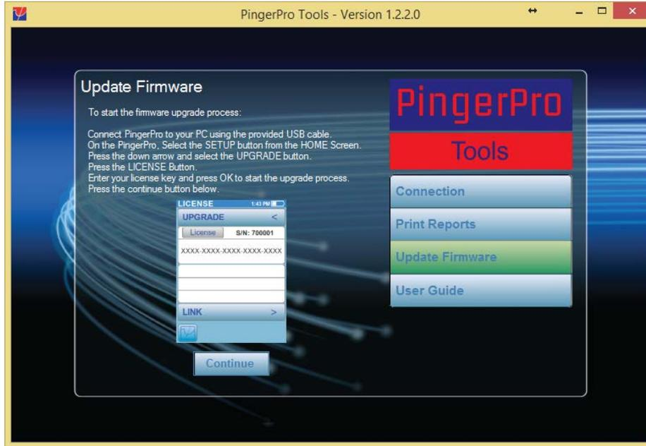
Select the **Update Firmware** button on the PingerPro Tools to access the firmware update wizard. The steps to update the firmware are displayed in sequence for a more descriptive upgrade experience. This same information can be found under the **Upgrades** section of this User Guide.
