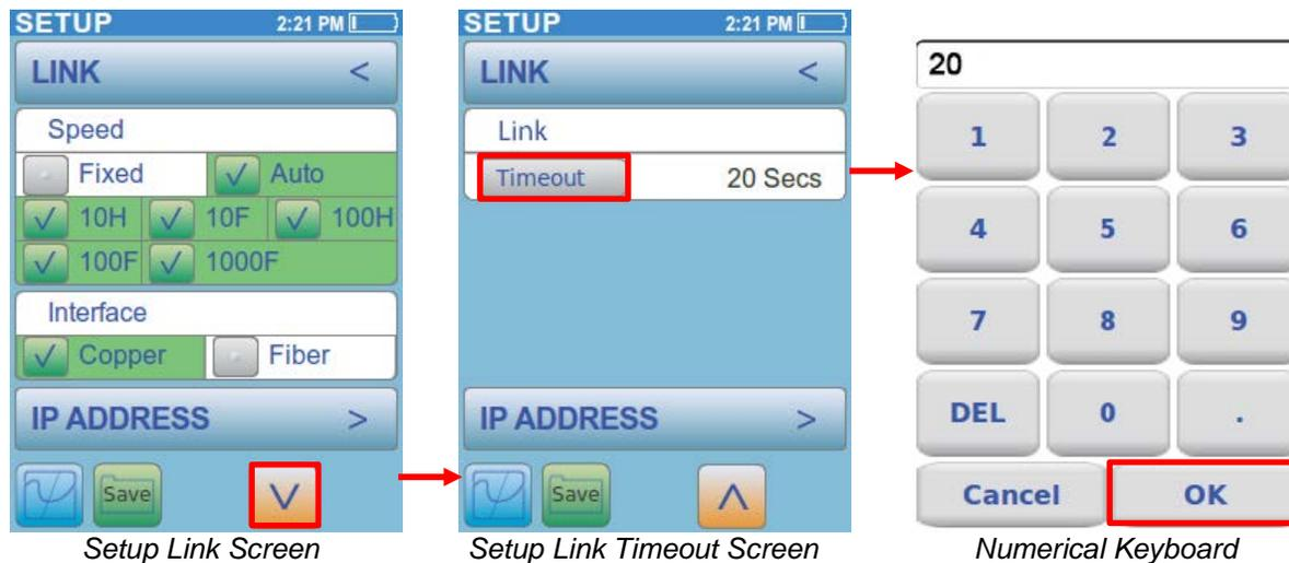
Select the **Link** button with the **<** arrow to return to the Main Setup Screen or select the **IP Address** button to continue to the IP Address Setup Screen.
