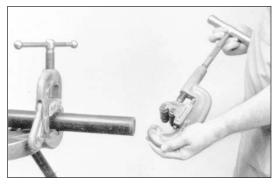
**A WARNING** Never try to cut pipe with the wrong cutter type or cutter wheel. This may result in serious injury and damage to the tool and work piece.
