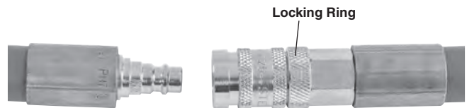
a. Loosen Locking Ring on Female Fitting
