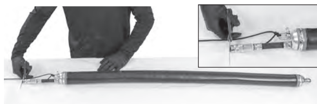
Figure 23 – Cutting Containment Tube To Length For Full Packer
