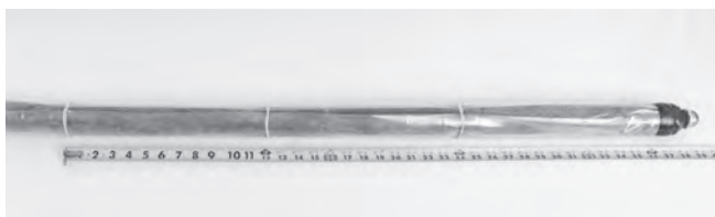
Figure 16 – Elastic Band Placement On Packer Sleeve (Every 12")
