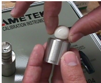
After the ball and nozzle have been cleaned, slide the ball through the nozzle. The ball should pass through the nozzle with no resistance.
