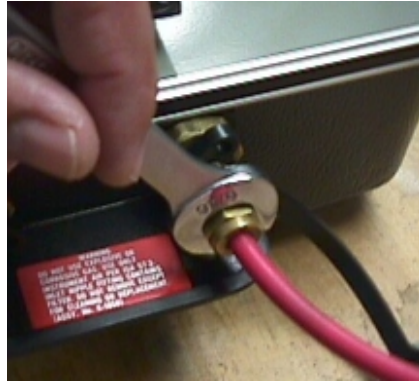
Connect clean, dry and oil-free air or nitrogen to the INLET valve.
