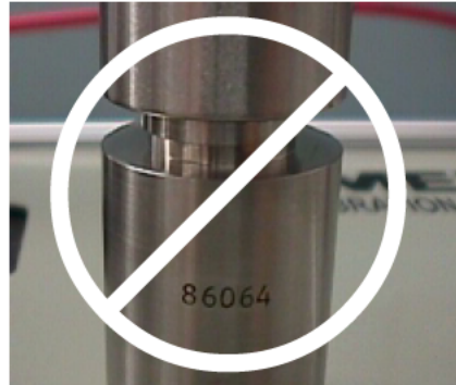
INCORRECT ALIGNMENT- The serial numbers DO NOT align and may lead to inaccurate readings.
