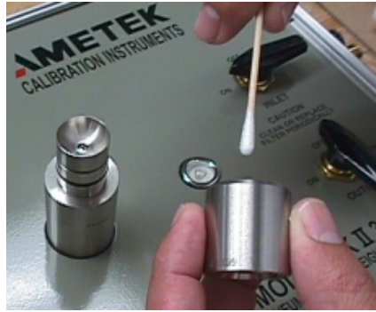
Using a cotton swab or soft cloth with a solvent such as alcohol, wipe the inside of the nozzle.
