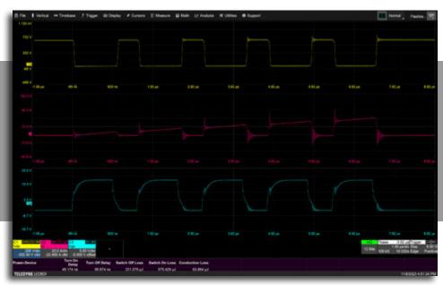
The Power-Device software option allows for simplified silicon carbide (SiC) and gallium nitride (GaN) analysis by automatically and accurately measuring captured double pulse test (DPT) waveforms.
