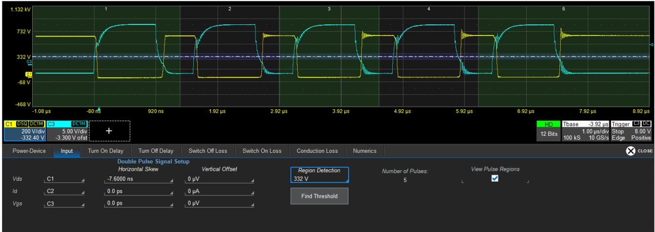
*By moving the marker to the Vds median level, the Number of Pulses identified is five.
