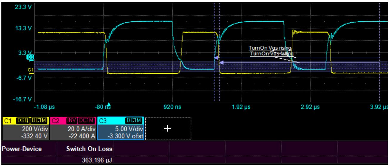
Or from the 99% falling edge of Vds to the 10% falling edge of Vds:
