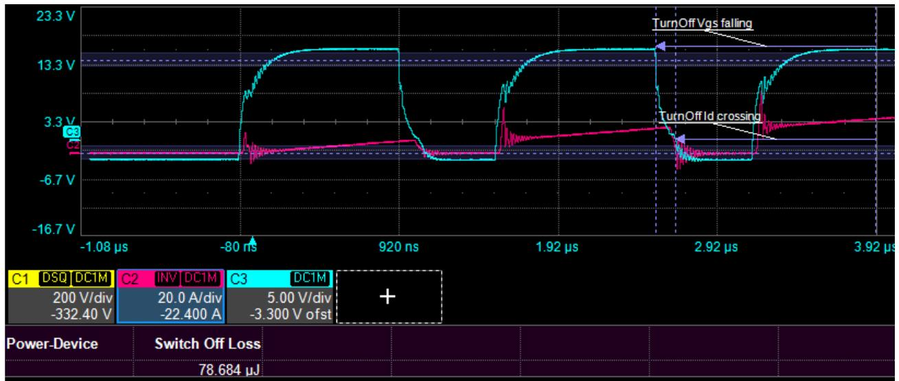
Or from the 1% rising edge of  $V_{ds}$  to the 0-crossing of  $I_d$ :
