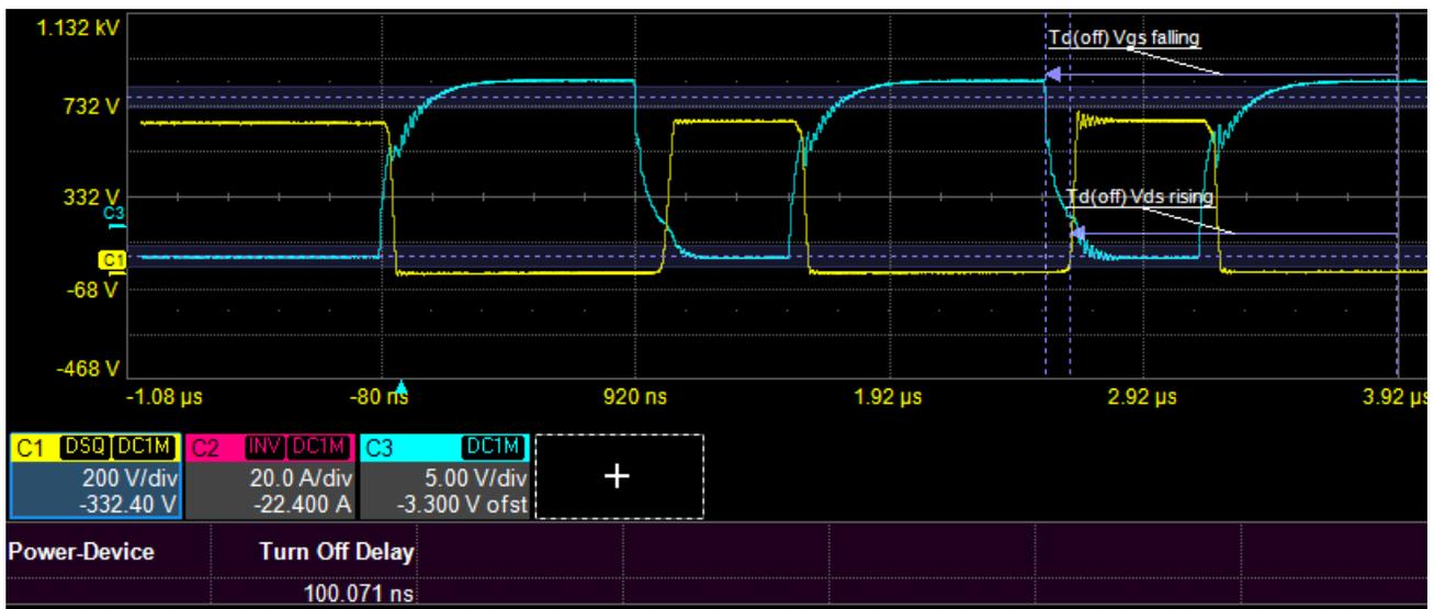
Or from the 90% falling edge of  $V_{gs}$  to the 90% falling edge of  $I_d$ :
