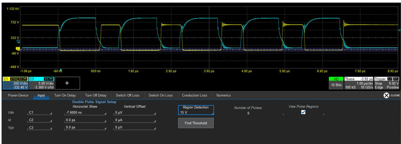
*The Number of Pulses is 0 because the pulse region marker is set at too low a level to register any pulses.*
