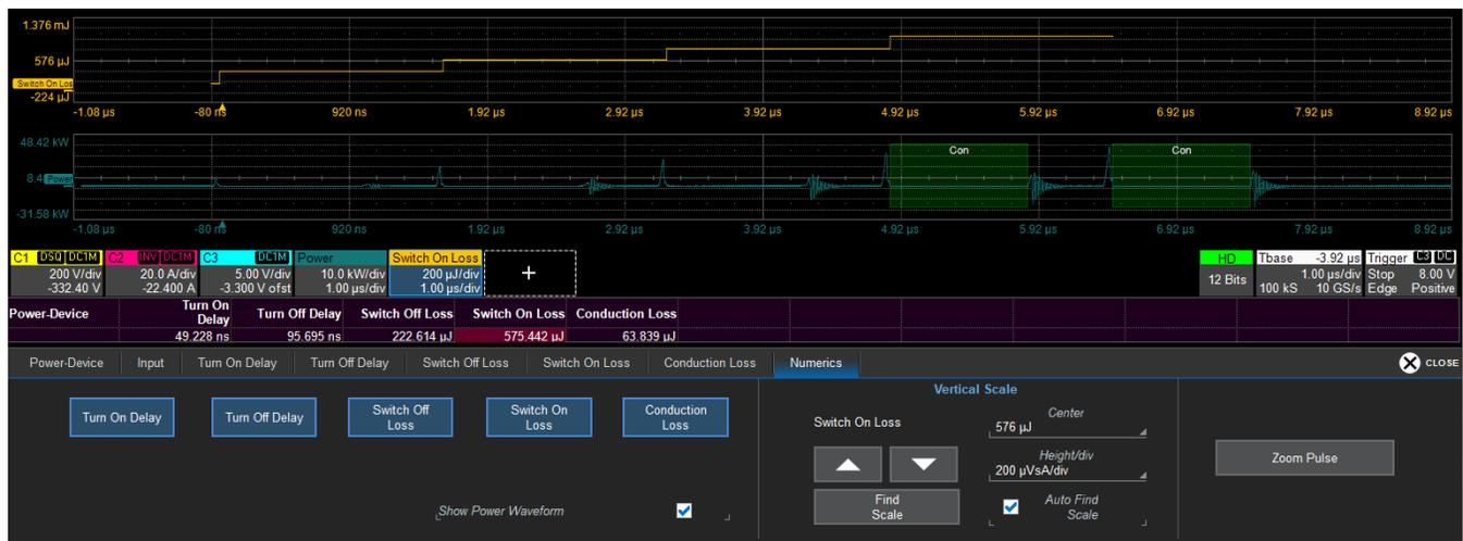
The power tracks are best used for measurements that are made on all pulses. Any spike in values will identify problematic pulses.
