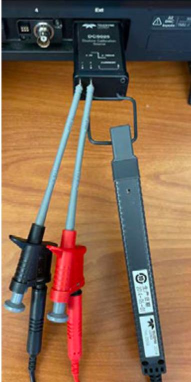
1. Connect a differential voltage probe to any open Channel ( $C_n$ ) input. On the voltage probe  $C_n$  dialog, select **Auto Zero**.
