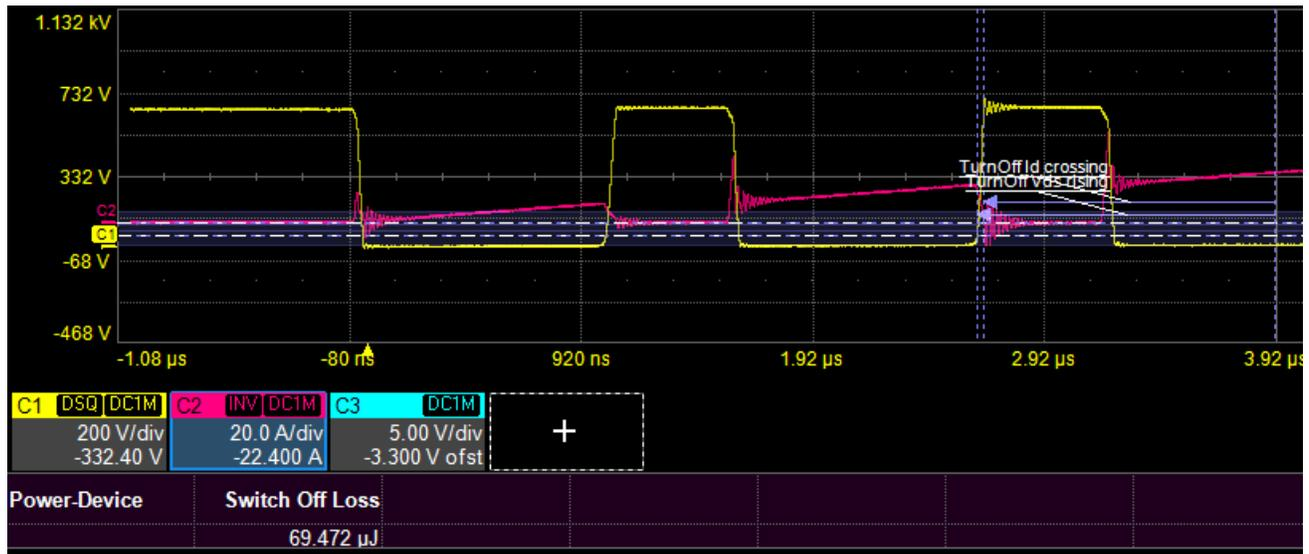
**Note:** The Switch Off Loss measurement may require manual adjustment to raise the threshold at which  $V_{ds}$  is measured. If you do not see a measurement at the Auto level, switch to Manual and drag the  $V_{ds}$  level marker up until you see a value in the table.
