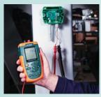
Precision "source" for calibrating process devices.
