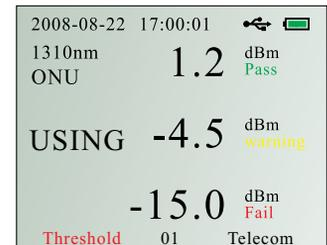
**Fig.3** Threshold Setup Menu
