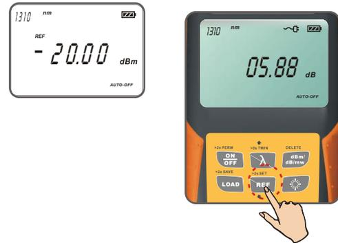
2. Press and hold the “REF” key over 2 seconds to store the presently measured value as the new reference level for the current wavelength. During the process the “REF” sign flashes twice on the screen and buzzer sound is heard. Once the new reference level is set, the instrument switches to the dB measurement mode. The displayed value only lasts 1 second.
