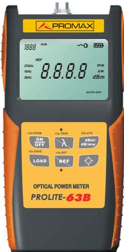
The **PROLITE-63B** are full featured palm sized optical power meters designed for use with an optical laser source to perform optical loss measurements on optical fiber cables. The **PROLITE-63B** are lightweight and are controlled by microprocessor. Utilizing state-of-the-art SMT in its manufacture, optical connections to the **PROLITE-63B** are made via the universal adapter interface on the top of the unit. The instrument has 6 working wavelengths to totally satisfy your needs.
