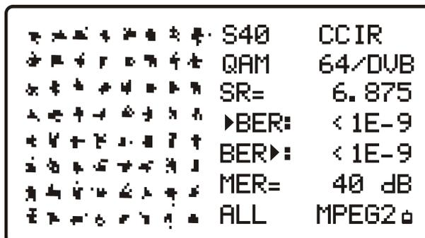
**Figure 22.** Constellation Diagram representation and Pre-BER, Post-BER and MER measurement in a digital channel.
