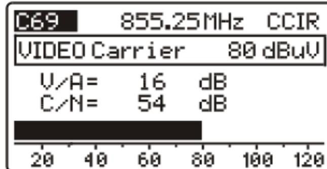
**Figure 15.** V/A and C/N Level measurement.
