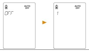
If the auto off time is set to be "Off", then the unit will not automatically turn off. Preserve battery life by lowering this setting to a minimum on time. A user must manually turn it off by pressing and holding the  $\bigcirc$  button for 5 sec.
