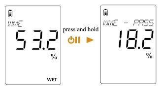
press key to exit the calibration check.
