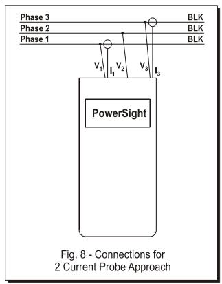
three-phase circuit. The disadvantage of this approach is that you cannot determine the power, power factor, or VA of each individual phase and, of course, you cannot record the current of one of the active phases.
