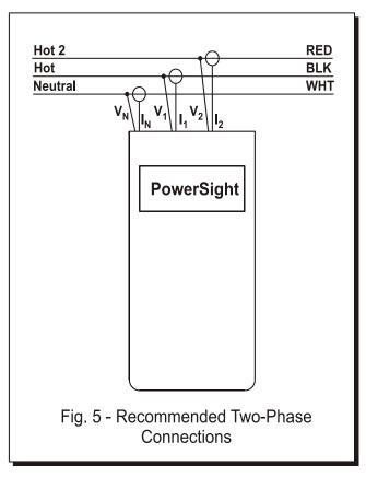
remove the V<sub>N</sub> voltage lead since it may affect the power factor readings of each phase.
