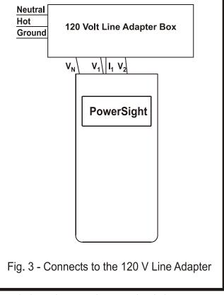
socket and then attach the voltage and current leads into PowerSight. Each lead is labeled to eliminate errors in connections.
