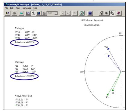
signal, so its angle is 0 degrees. If the phase 1 current lags it, it will be slightly above it. In a three phase circuit, normally the other two phases will be 120 degrees before and after phase 1 and the phase lag of each current relative to its associated voltage will be similar. The data graphs on the left of the phasor display show the actual degrees of all voltages and currents in relation to the phase 1 voltage and show the phase angle between the voltage and current of each phase.
