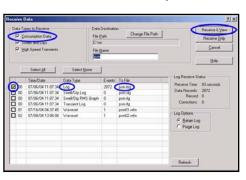
of the file is based on the entry in the File Name box. For instance if "psm" is entered in the File Name box, the consumption log will be called psm.log. If you want a different root name, change it before receiving the file.
