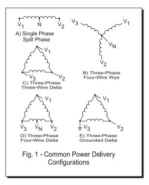
(240V) is used by delivering both hot voltages to the load. Neutral provides the current return path. If the load is balanced, there will be relatively little neutral current. Refer to figures  $\underline{2}$ ,  $\underline{3}$ ,  $\underline{4}$ , and  $\underline{5}$  for various ways to connect to single-phase and split-phase power service.
