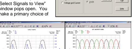
voltage, current, or voltage and current and then you make a secondary choice of which phase or phases to view, then click on "OK".
