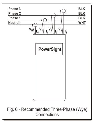
Although the current of each phase is carried by neutral, neutral current is generally relatively small since the currents of the 3 phases largely cancel each other in the neutral leg. In a perfectly balanced system the current in neutral would be zero.
