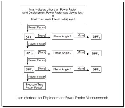
says "Displacement P.F.". The sequence of the display is DPF<sub>1</sub> > DPF<sub>2</sub> > DPF<sub>3</sub> > TPF<sub>1</sub> > TPF<sub>2</sub> > TPF<sub>3</sub> > TPF<sub>T</sub>.
