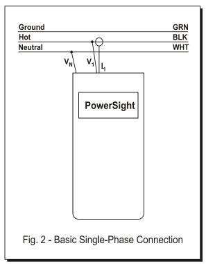
Since voltage now comes into PowerSight on V<sub>1</sub> and current is sensed by I<sub>1</sub>, the power and power factor for this single-phase system will be available as phase 1 power and phase 1 power factor.
