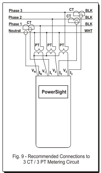
its rating plate. A typical value would be 600:5 (120:1). The output of each CT must have some burden across it for the secondary current to flow. The current probes of PowerSight are clamped around the secondary of each CT. Make sure to use current probes that are suited for accurate measurement in the 0-
