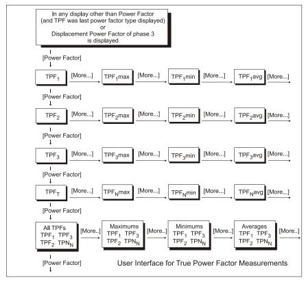
In this way, by combining the [Power Factor] and [More...] keys, there are 16 true power factor measurements available.
