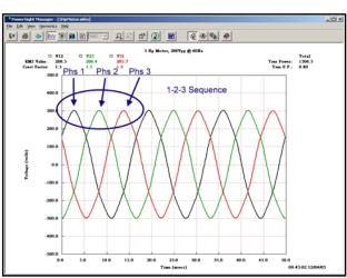
waveform will be followed next by the highest level of the  $V_{2N}$  (or  $V_{23}$ ) waveform, which will be followed by the highest level of the  $V_{3N}$  (or  $V_{31}$ ) waveform (see the example).
