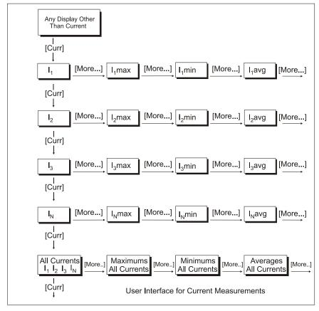
For instance, if the average current of Phase 3 is desired, press: [Current] (to display I<sub>1</sub>), [Current] (to display I<sub>2</sub>), [Current] (to display I<sub>3</sub>), [More...] (to display maximum I<sub>3</sub>), [More...] (to display average I<sub>3</sub>). Following
