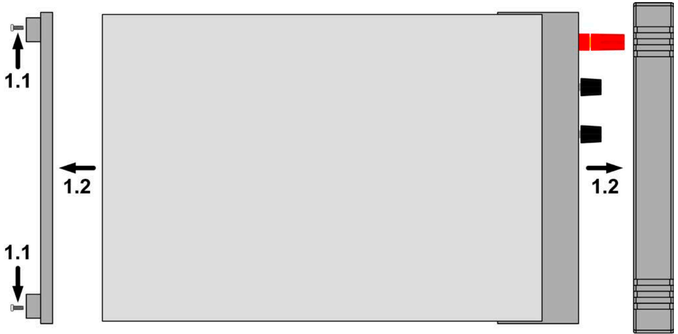
Figure 8 - Removal of the front and rear frame
