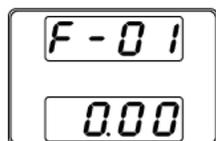
3. Rotate the Voltage knob to change the F setting to F-89 (Show Version).
