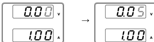
3. Repeatedly press the Voltage knob until the first digit is highlighted. This will allow the voltage to be edited in 1 volt steps.
