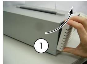
2. Remove the filter from the grill and replace with a new filter (GW Instek part number PSW-010).
