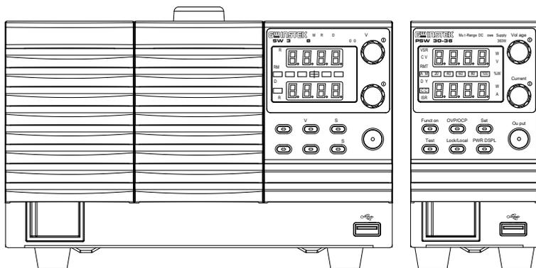
**Function Keys**      The Function keys along with the Output key will light up when a key is active.
