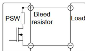
Bleed resistors are designed to dissipate the power from the power supply filter capacitors when power is turned off and the load is
