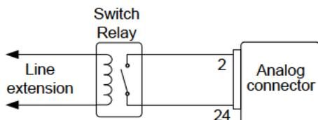
If a single switch control is to be used for multiple units, please isolate each instrument. This can be achieved by using a relay.
