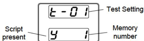
3. Rotate the Voltage knob to change the T setting (Test setting).
