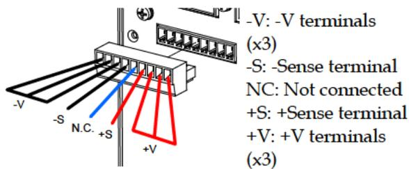
**Wiring the Connector Plug**
