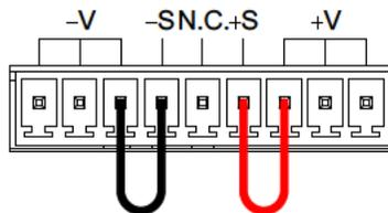
7. If not using local sense, see the remote sense section to wire the sense terminals for remote sensing. Page 71
