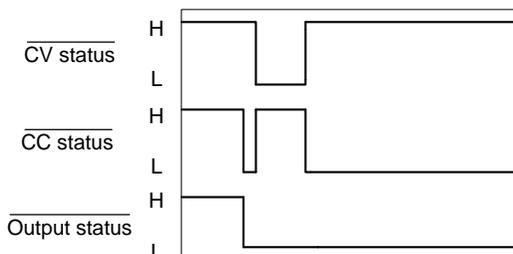
CC MODE: The diagram below shows the output status lines
