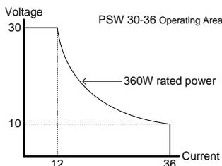
When the power supply is configured so that the total output (current x voltage output) is less than the rated power output, the power supply functions as a typical constant current, constant voltage power supply.
