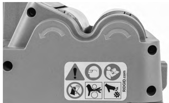
Figure 5 – Roller Direction of Rotation
