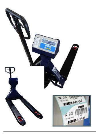
Offering an all-in-one solution, the PTT Pallet Truck Scale combines the power of a 5000lb/2000kg capacity heavy-duty pallet truck scale with the convenience of a built-in label printer. The PTT features solid steel pallet forks, wheels that swivel for easy movement and an audible alarm that indicates when capacity is exceeded.
