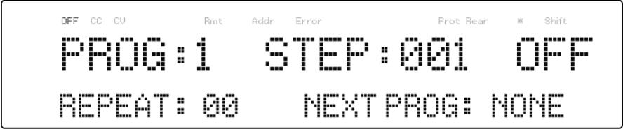
7. At this point, the user may select how many times they wish the current program to repeat in the **REPEAT** field, by using the keypad or the rotary knob.
