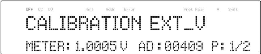
The *P: 1/2* signifies there are 2 points to be calibrated and the current calibration point is 1.
