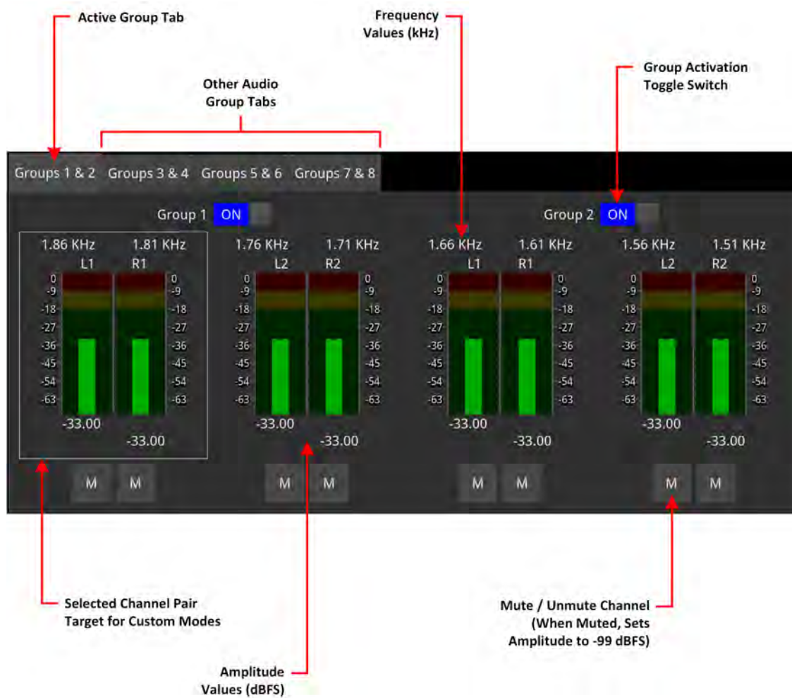
Figure 6-25: Audio Generator Configuration Dialog - Audio Group Selection Panel
