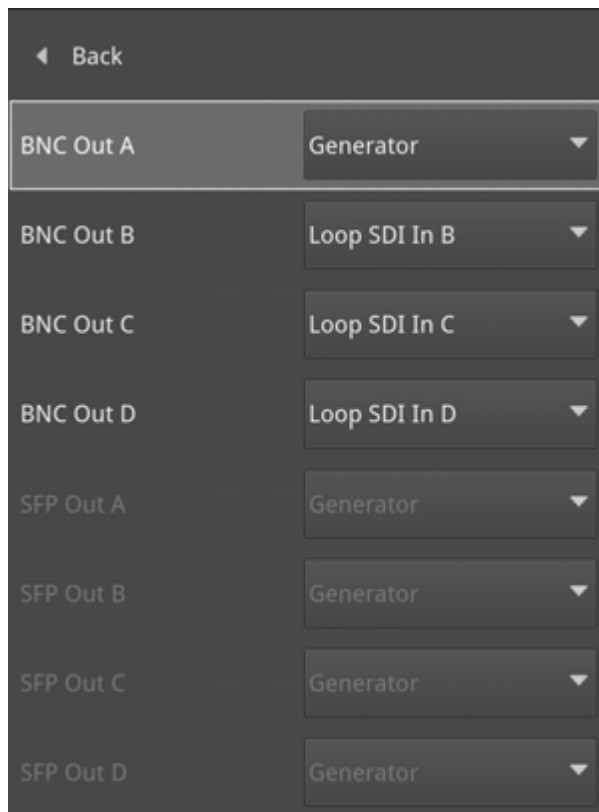
Figure 6-19: Generator - SDI Output Assignment
