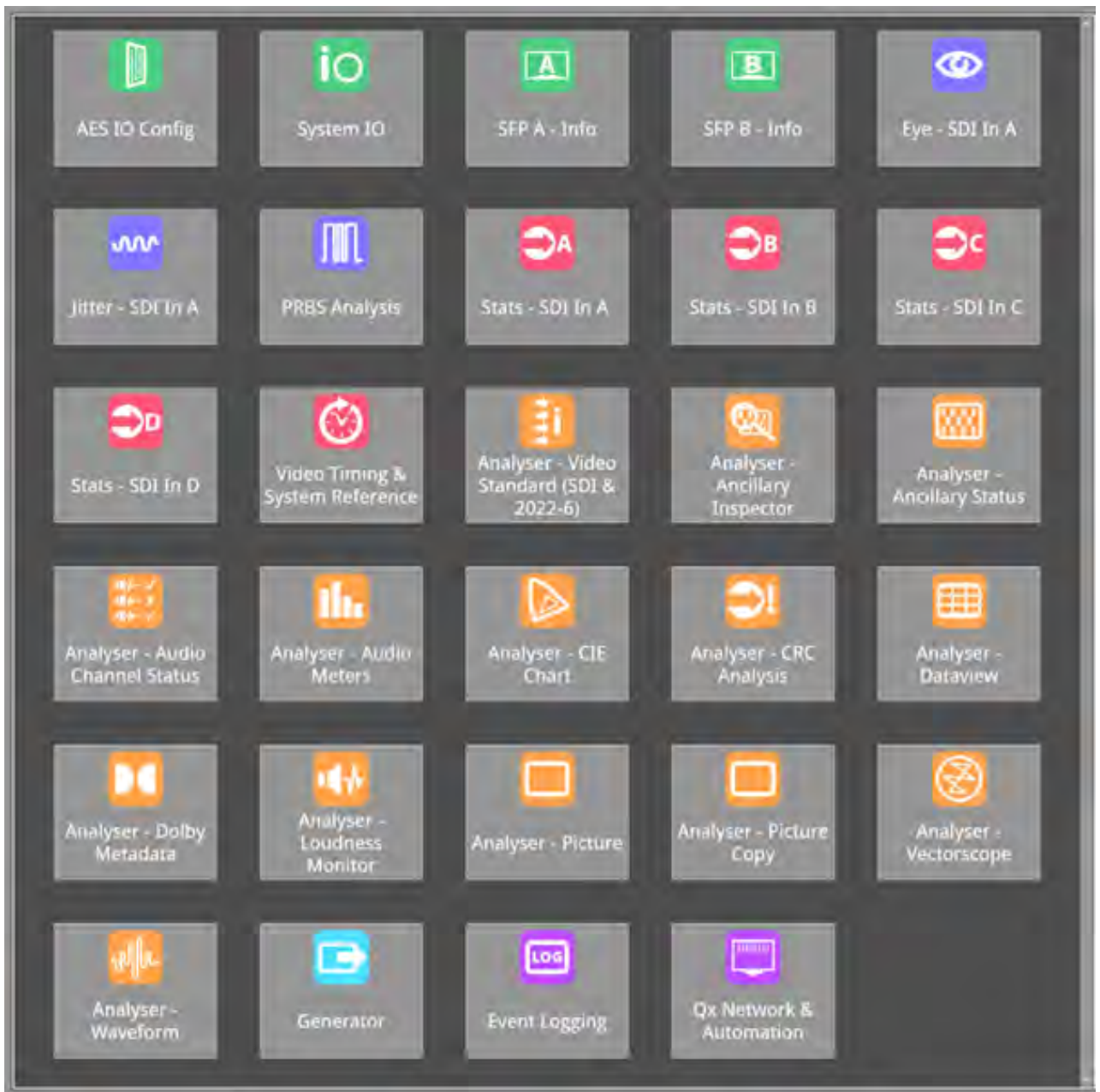
Figure 2-12: Instrument Panel in SDI Boot Mode (Factory-fitted Option)
