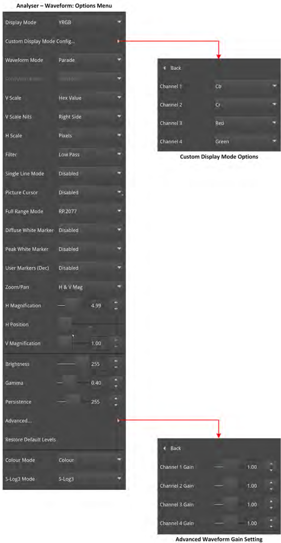
Figure 9-23: Analyzer - Waveform Options Menu and Submenus
