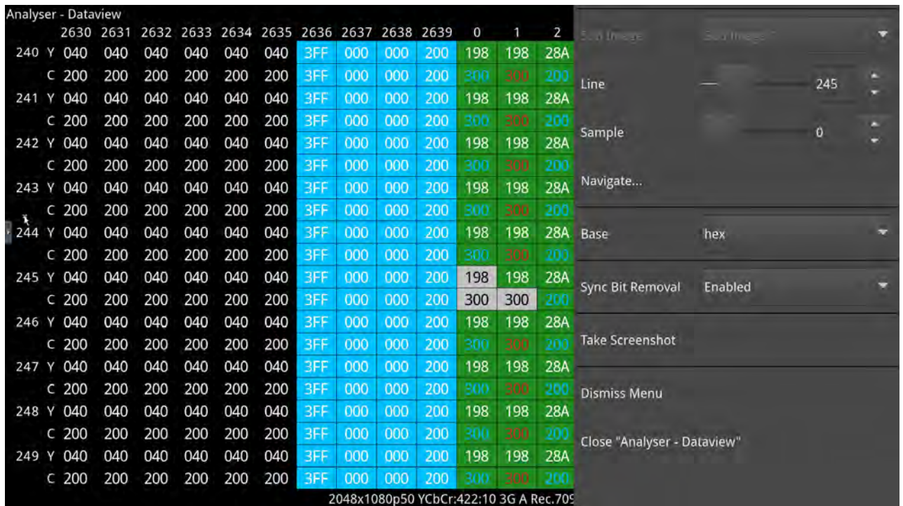
Figure 11-1: Analyzer - Dataview Instrument
