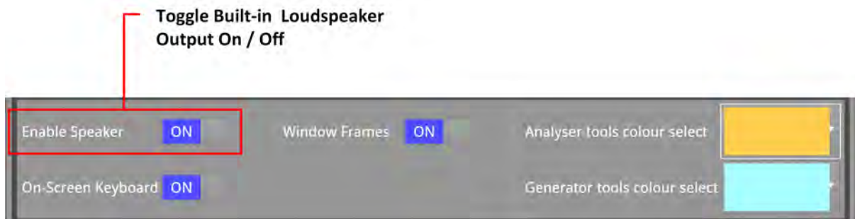
Figure 2-20: Enabling the Built-in Loudspeaker in the Settings Dialog
