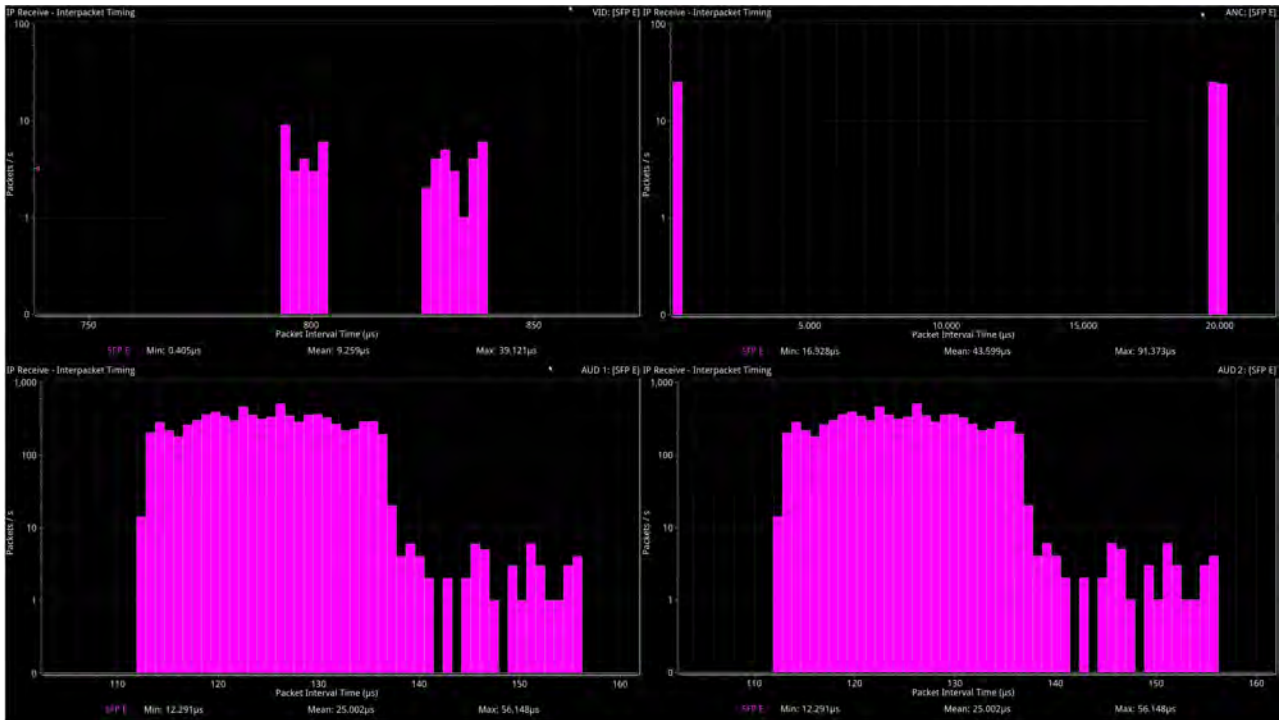
Figure 12-2: IP Receive - Interpacket Timing in IP 2110 Boot Mode
