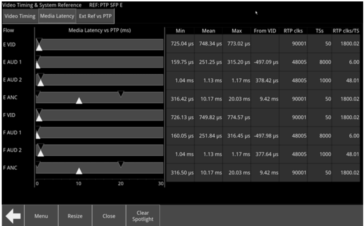
Figure 12-10: Media Latency Tab of the Video Timing & System Reference Instrument (IP 2110 Boot Mode)
