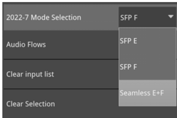
Figure 12-4: SMPTE ST 2022-7 Mode Selection of Seamless E+F in IP Receive - Flows
