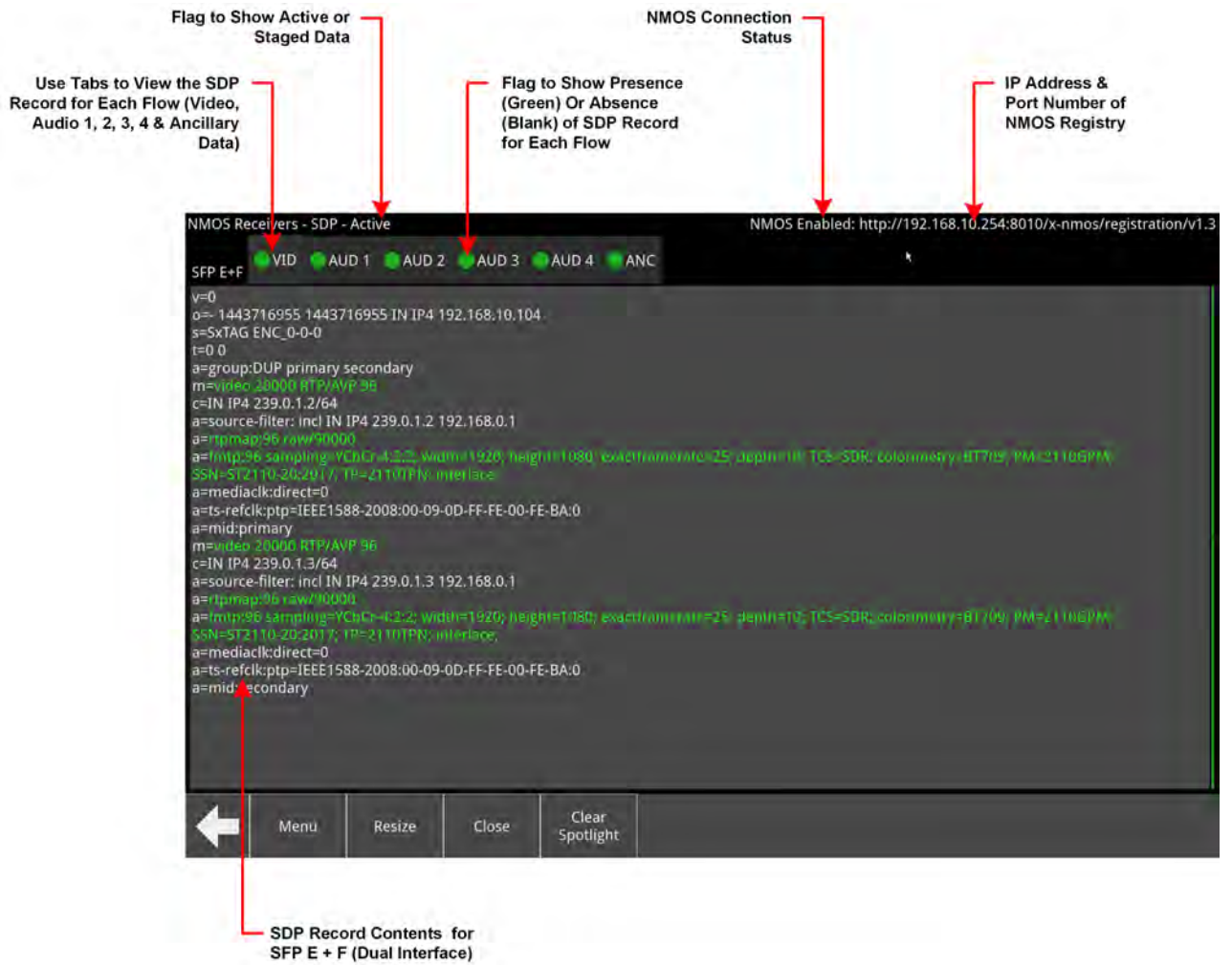
Figure 4-16: NMOS Receivers - SDP Instrument Views (Dual Interface, Full Screen Size) (IP 2110 Boot Mode)
