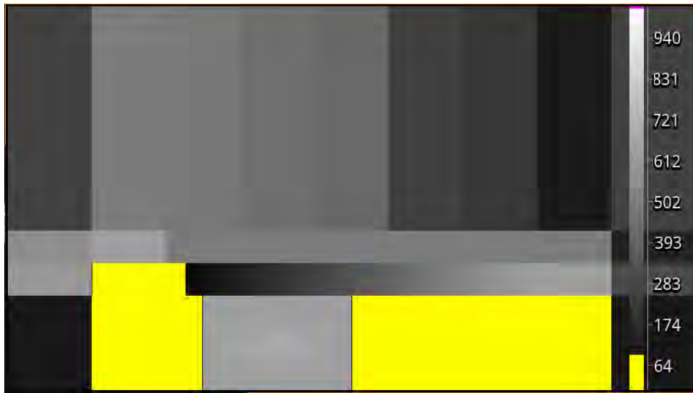
Figure 15-4: False Color Overlay Applied
