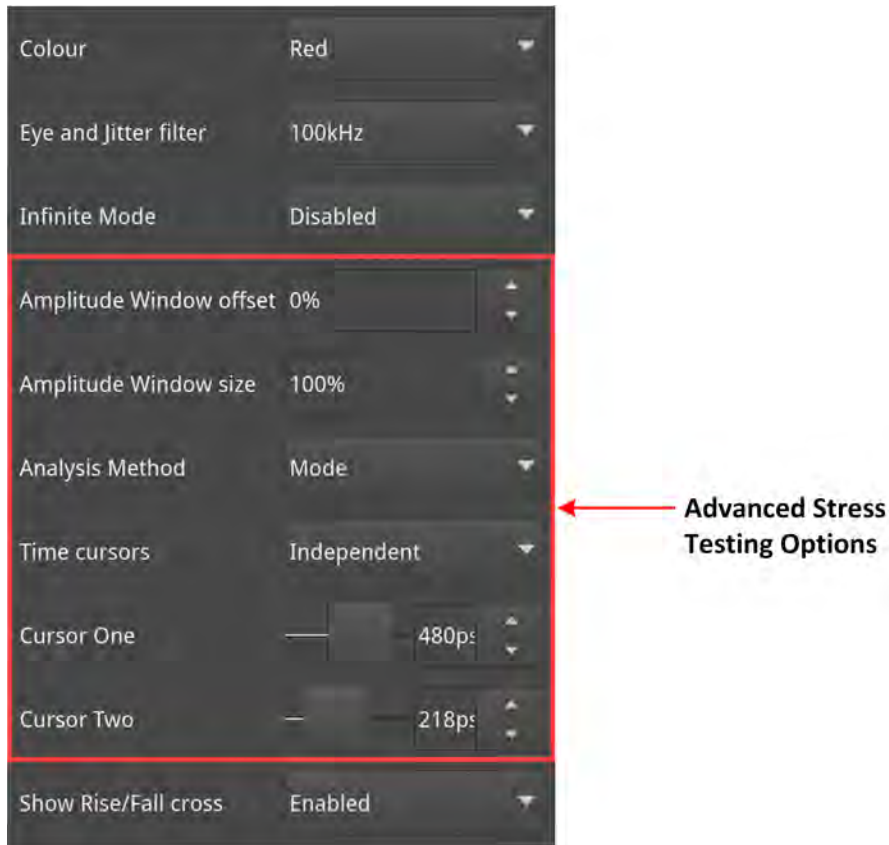
Figure 14-5: Eye - SDI In A Menu Showing Advanced Stress Testing Options
