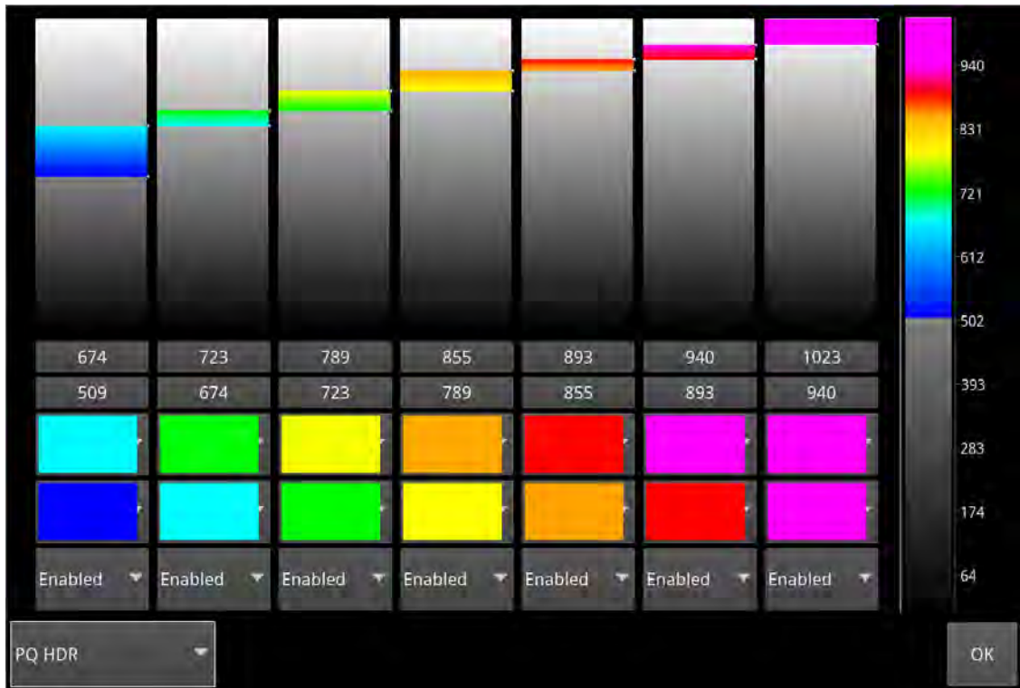
Figure 15-3: Configuring the False Color Overlay
