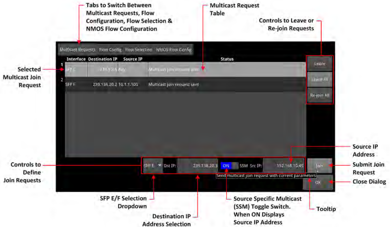
Figure 4-33: IP Receive - Flows: Multicast Requests Tab
