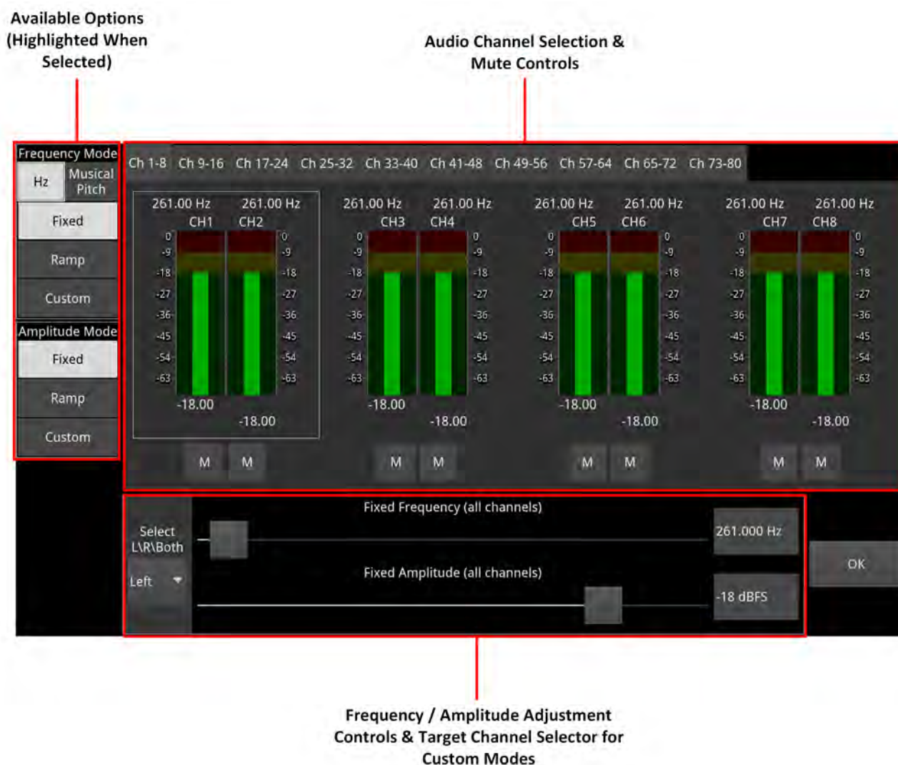
Figure 6-27: Audio Generator Configuration Dialog (IP 2110 Boot Mode)
