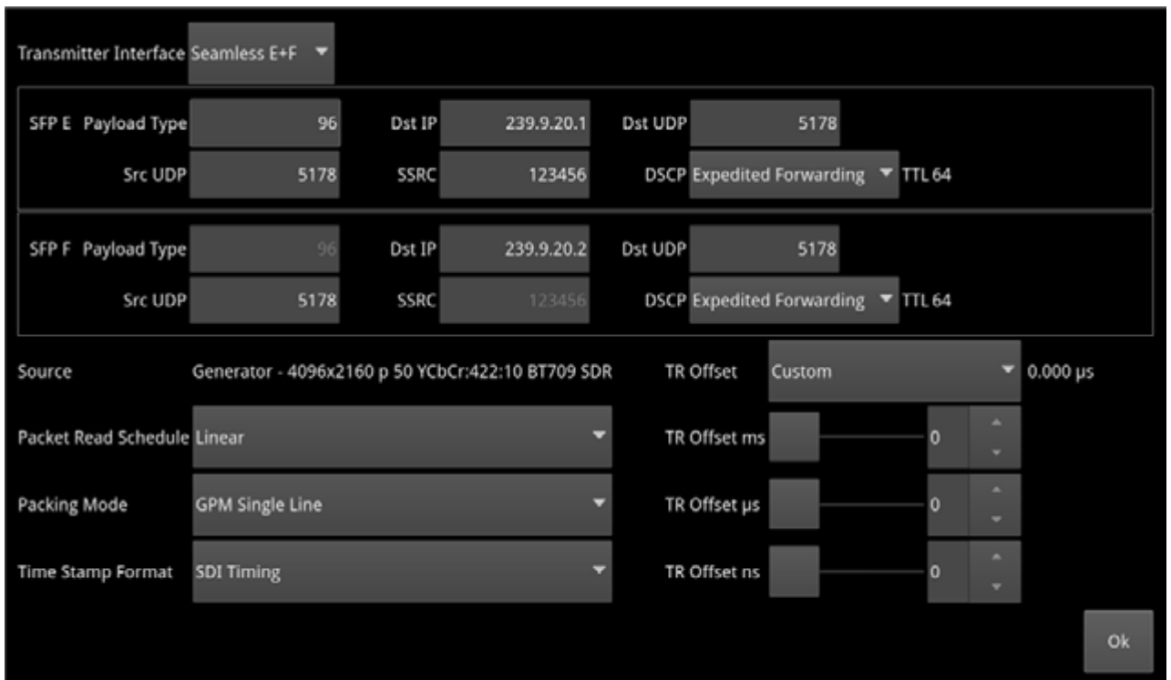
Figure 6-41: IP Transmit - Generator Video Flow Configuration
