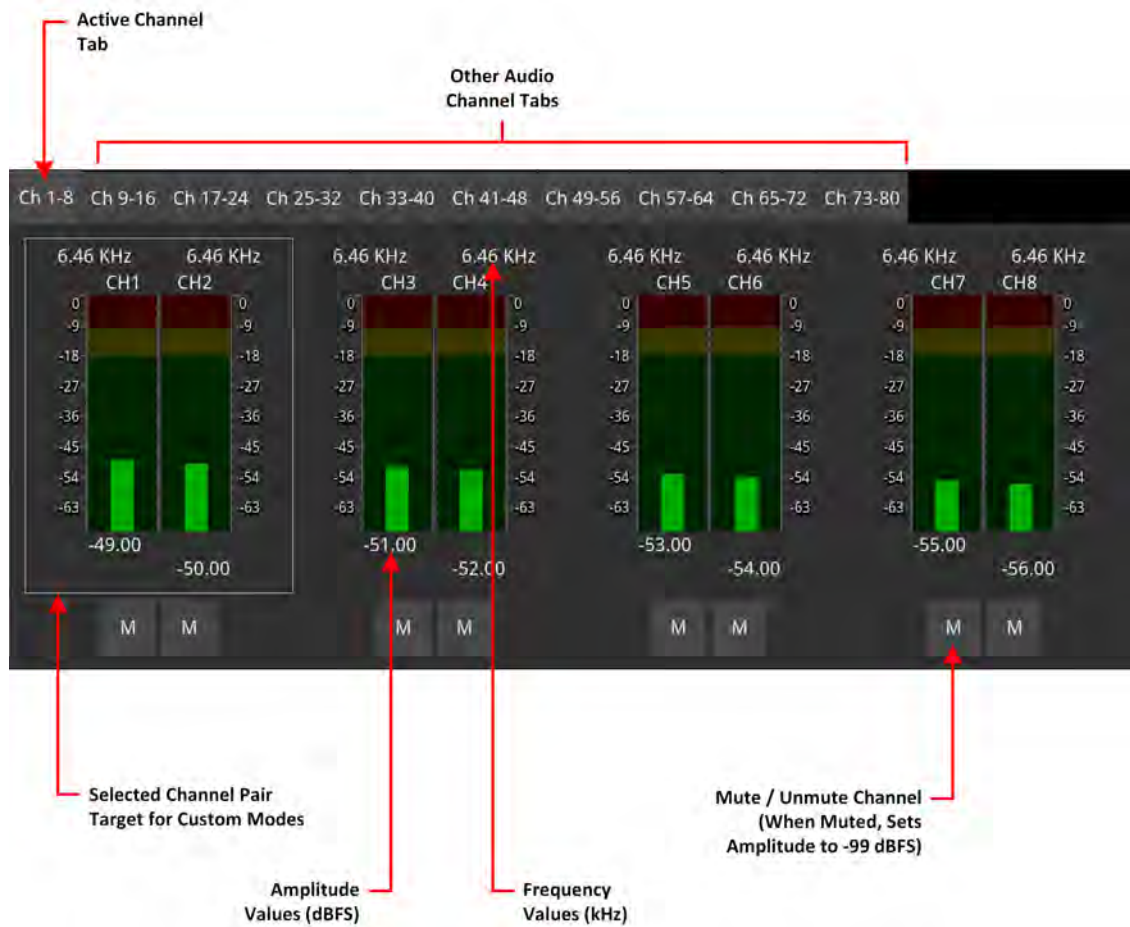
Figure 6-29: Audio Generator Configuration Dialog - Audio Channel Selection Panel
