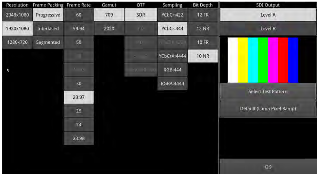
Figure 6-5: Generator Video Configuration (IP 2022-6 Boot Mode)
