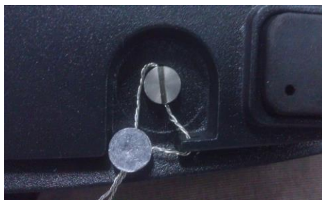
Locked with Wire Seal
