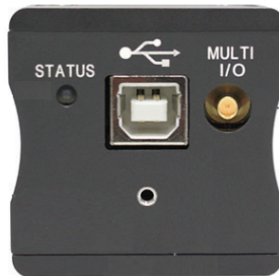
Figure 2.1 USB Connector and Status LED
