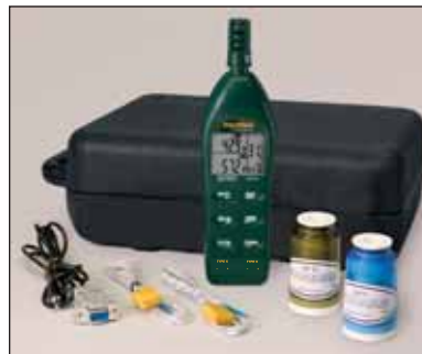
RH355 Superheat Psychrometer Kit includes meter, 33% and 75% calibration bottles, 2 temperature probes, RS-232 cable, 4 AAA batteries and carrying case.
