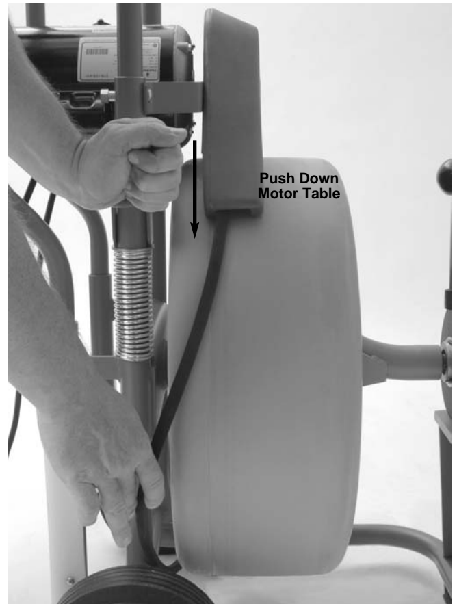
Figure 17 – Releasing Belt Tension
