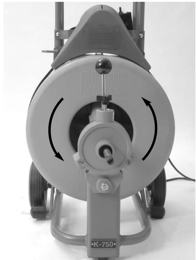
Figure 8 – Proper Drum Rotation (FOR Switch Position)
