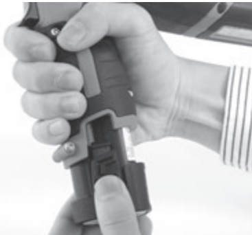
Figure 8 – Installing/Removing Battery In Tool
