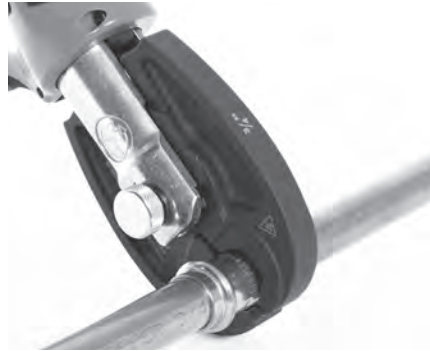
Figure 9 – Placing Jaws Around Fitting
