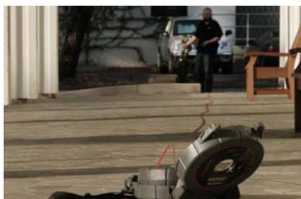
3. Using both hands, begin to rewind the push cable into the drum. If the push cable cannot be laid out straight, use extreme care when rewinding the push cable. Ensure the push cable does not bend or get caught on or under objects.
