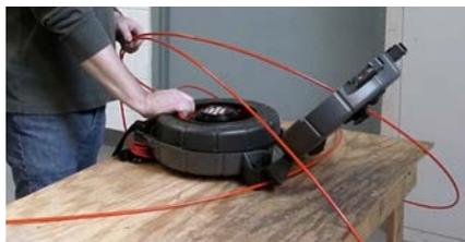
2. If space permits, uncoil and straighten the entire length of push cable on the ground.
