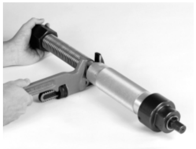
Figure 1 – Assembling Valve Adapter Onto Feed Screw
