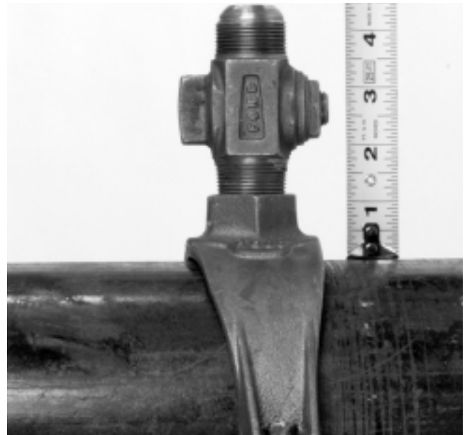
Figure 7 – Measuring Valve Stand-Off Distance – Minimum Stroke
