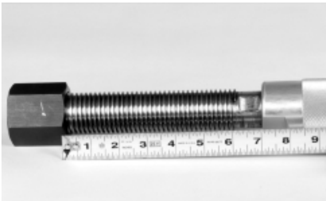
Figure 6 – Measuring Full Stroke Distance
