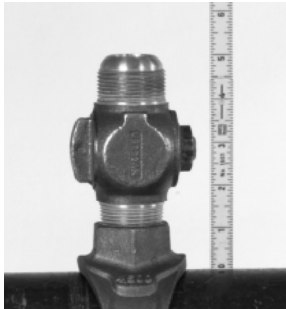
Figure 8 – Measuring valve standoff distance
