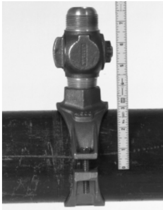
Figure 9 – Measuring valve standoff distance
