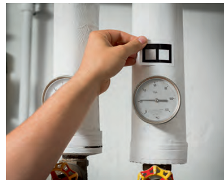
Attach ε-marker and record the object with the digital camera in the thermal imager.
