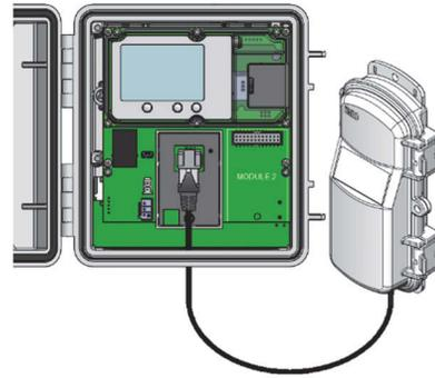
7. Plug in the battery and charging device, and wait for the device to power up. Verify that the new module is listed on the LCD screen with a checkmark.
