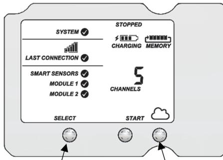
Press the Select button to return to the main LCD screen      Press the Connect button
