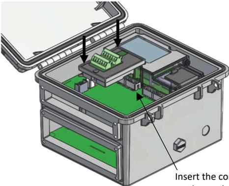
Insert the connectors on the module here
