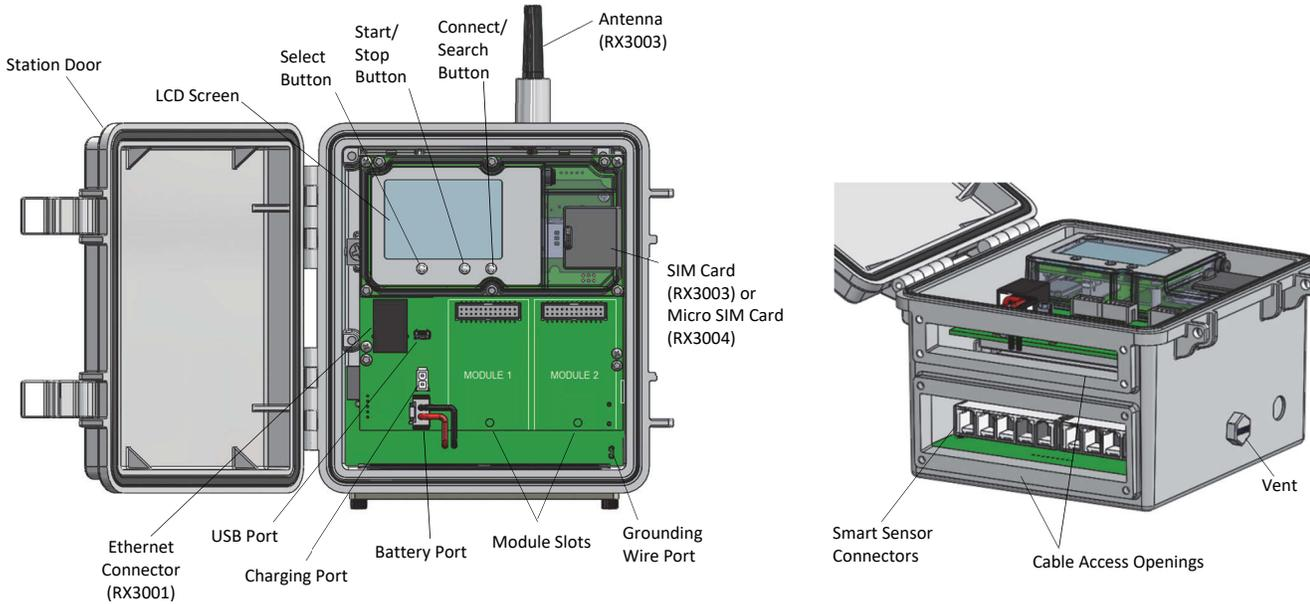
**Station Door:** This is the protective, hinged door covering the LCD and electronics. The station serial number and device key needed for HOBOLink registration are located on the inside of the door.
