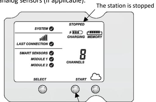
2. To stop logging, press the Stop button. Logging stops immediately. Note that the station will continue to connect to HOBOLink even if it is not logging.
