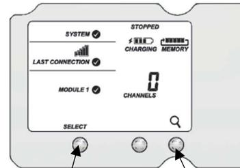
Press the Select button to switch to the module with RXW Manager installed      Press the Search button for the station to search for motes to join
