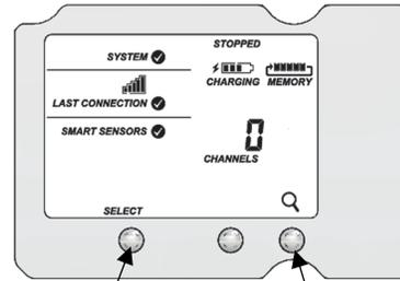
Press the Select button to view the smart sensor screen      Press the Search button for the station to find all connected smart sensors
