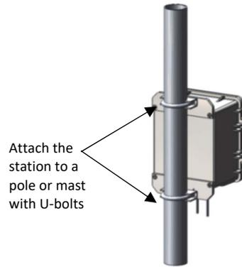
Attach the station to a pole or mast with U-bolts
