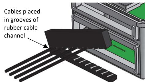
Cables placed in grooves of rubber cable channel
