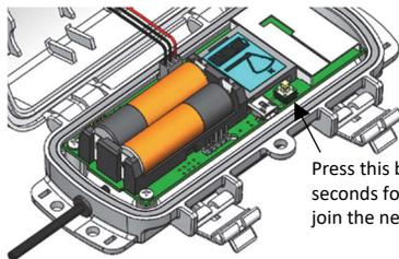
Press this button for 3 seconds for the mote to join the network
