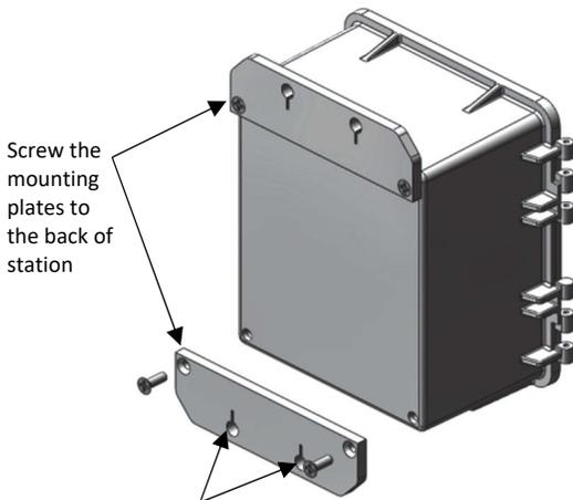
Screw the mounting plates to the back of station
