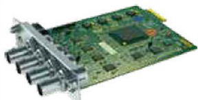
PHRXM-4 AES Audio I/O 75 Ohm unbalanced
