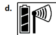
Once the mote has finished joining the network, the "x" icon is removed and the channel count on the station LCD increases by two (one for leaf wetness and one for the mote battery).
