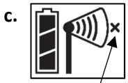
This network connection "x" icon blinks while the mote completes the registration process, which may take up to five minutes.
