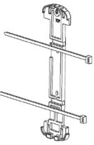
Insert the bottom of the sensor node into the retaining clips on the bottom of the bracket then press the top of the sensor node into the clips at the top of the bracket.
