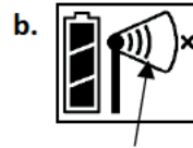
Once a network is found, the icon will stop flashing and the bars will cycle from left to right.
