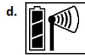
Once the mote has finished joining the network, the "x" icon is removed and the channel count on the station LCD increases by two (one for the pulse input sensor and one for the mote battery).
