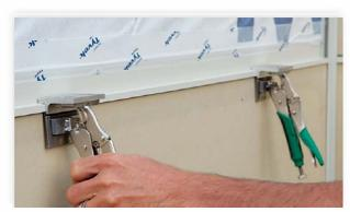
To adjust siding-to-flashing gap, simply remove or add the included spacer plates. Sliding the spacer plates forward adjusts for the siding thickness, while the tension knob adjusts for flashing thickness.
