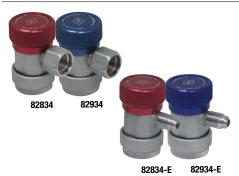
Patented manual couplers adjust easily to R134a service ports with varying dimensions. All metal construction for extra durability. Patented, spring loaded depressor will not damage service valves. Can be removed from service ports regardless of knob position without losing refrigerant. Meets SAE, UL and EPA requirements for containment of refrigerant. Color coded. **PATENT# 5,370,359**
