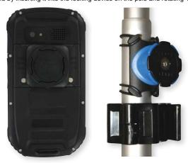
Once the handheld is attached to the pole, the SMART Air Hood® balancing instrument is now ready for use.
