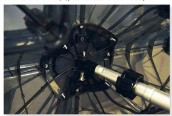
When using the short pole or with the SAH adapter base kit for canvas hoods, the stationary pole adapter should be used to keep the hood pole from pivoting. Place the stationary pole adapter onto the SAH and attach using the screws and wing nuts provided (below). Once secure to the SAH, insert the short pole and secure in place using the locking pin.
