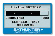
but 70% of the total battery capacity is recovered in the first hour thanks to Li+ technology. Using the adapter cable shipped with **SATHUNTER+**, the equipment can be charged from a vehicle's cigarette lighter in route to jobs.
