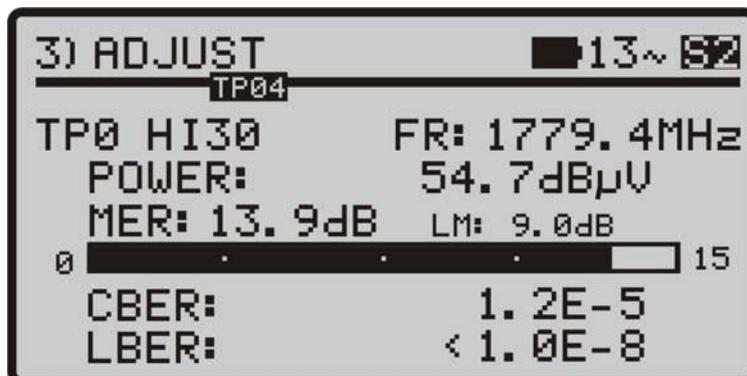
**Figure 15.- DVB-S2 measurements with LBER.**
