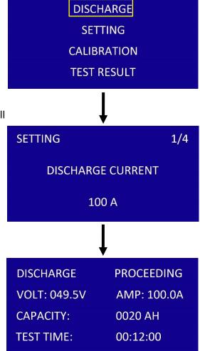
**6.5** During discharge, press the to go back to parameter settings, change the settings values by then press to apply the new settings and continue the discharge.
