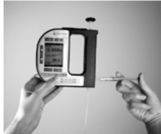
Fig. 10 - 2 Filling sample using the plastic syringe
