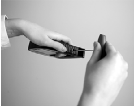
Fig. 12 - 2 Removing the pump lock screw
