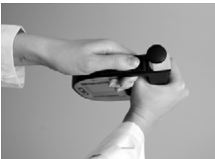
Fig. 12 - 1 Removing the pump
