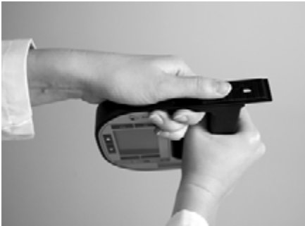
Fig. 12 - 3 Removing the pump lock
