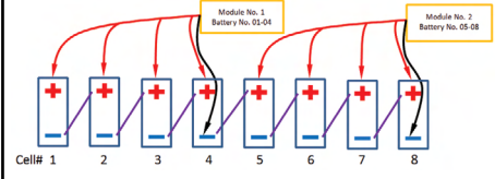
Monitoring 1.2 or 2V Cells with 1.2/2V Module
