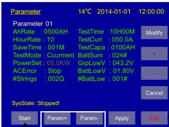
Press “Modify” to locate the preset parameters needed to be changed, “+”, “-” to change value, “Cancel” to quit. After desired values are entered, press “Apply” to save, and **the desired changes will be updated to “Preset”**
