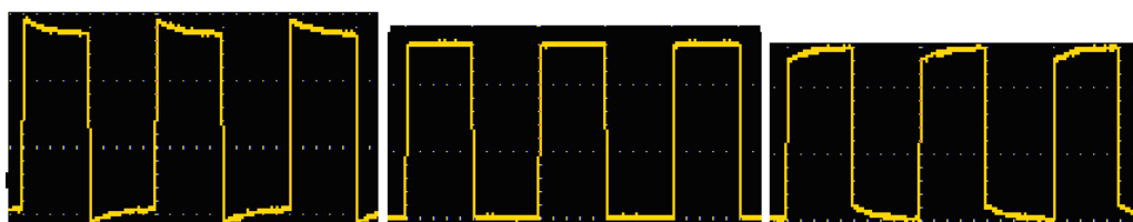
Figure 3-6 Displayed Waveforms of the Probe Compensation
