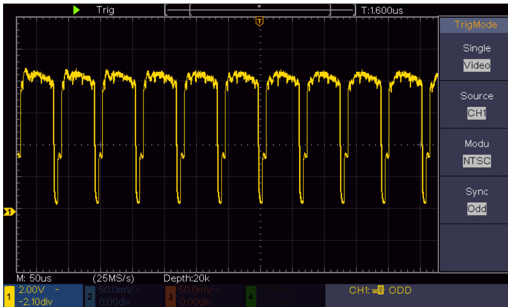
Figure 6-7 Waveform Captured from Video Field Trigger
