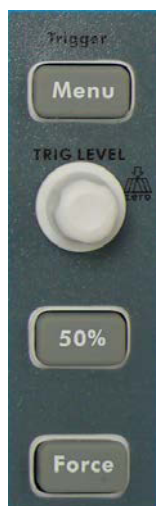
Figure 4-13 Trigger Control Zone
